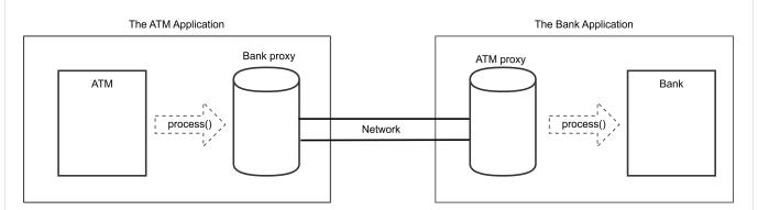
At this point, the ATM needs to send a message to the Bank object, asking it to process a transaction (passing the Withdraw transaction object as an explicit argument). The ATM object lives in one address space (the ATM application) but the Bank lives in a different address space (the Bank application). We will employ proxies to make the ATM and the Bank objects viewed in the same address space.
